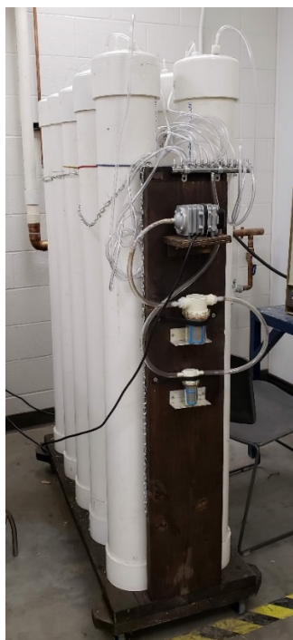
Figure 2: Reactor set up using schedule 40 PVC tube and cap, and ventilation system, for long-term additive test.
