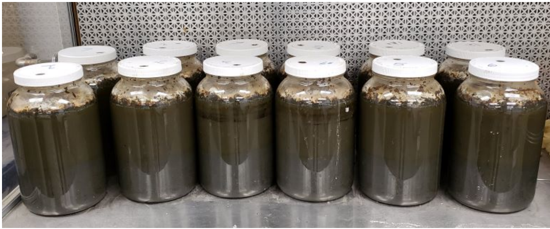
Figure 1: Semi-long-term pit additive test, with 12 glass jars set up in laboratory
